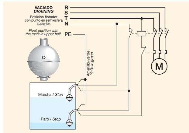
The level switches are supplied with the float in filling position, when the mark is shown on the lower hemisphere of the float. In order to operate for draining, the mark on the float should be situated in an inverse position on the upper hemisphere of the float. To do this has to remove the inferior lock washer of its slot, turn the float upside down and fit again the lock washer.
